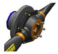
At this point, the propeller is installed on your aircraft with the spinner mounting plate.
