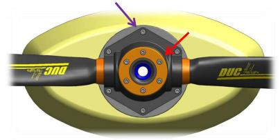
Slightly untighten the **propeller fixing screws** and the **hub assembly screw**.
